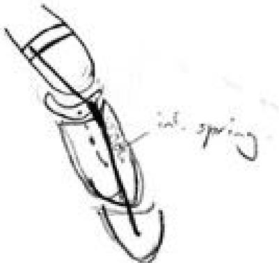
**Figure 3.** This design incorporates both a push/pull design centered on a ring the patient wears and a lever mechanism resting on the anterior surface of the amputated finger. By use of a moment arms the device will be able to flex based on the patient's articulation of their finger. The design features a built in spring to assist with extension of the finger following flexion.
