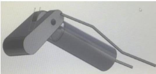
**Figure 2.** The wires depicted in this design attaches to a ring just below the proximal joint of the residuum of the finger. The rod will be directly attached to a cap covering the residuum. As the proximal joint bends, the force from the wires creates a moment in the lever acting as the distal phalanx. This leverage causes the device to bend downward, and the subsequent extension of the proximal joint will in turn cause the lever to extend.
