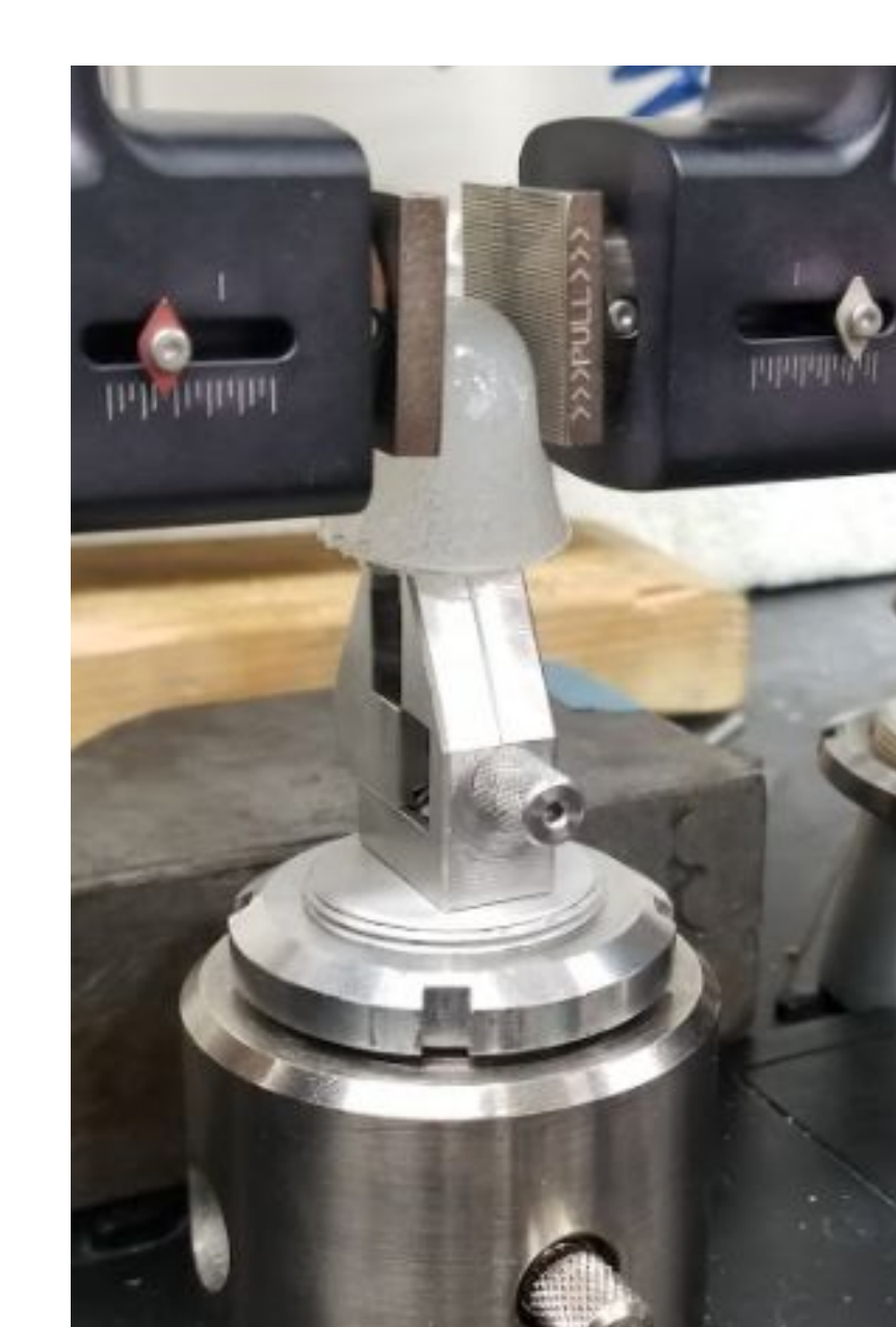
Figure 14: Silicone prototype undergoing testing in the MTS machine
