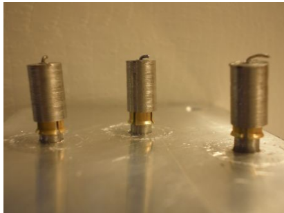
Figure 1. Spring and sheath design intended to replace the entirety of the magnet.
