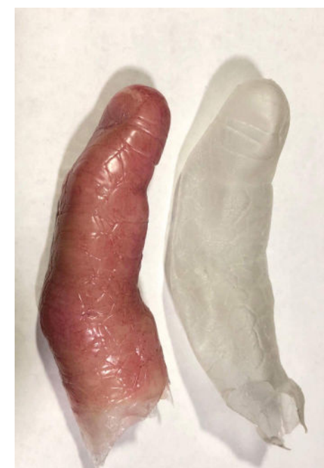
Figure 2: Attempted lining of silicone with PU sheath
