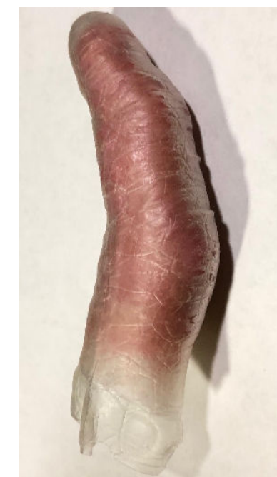
Figure 3: PU lining on the silicone prosthesis.
