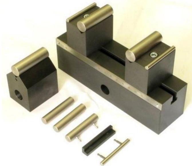
**Figure 8.** Image of three point bending fixtures similar to those used in the three point bending setup. The block to the left is the moving crosshead that applies a downward force, while the sample rests lengthwise on the part to the right.
