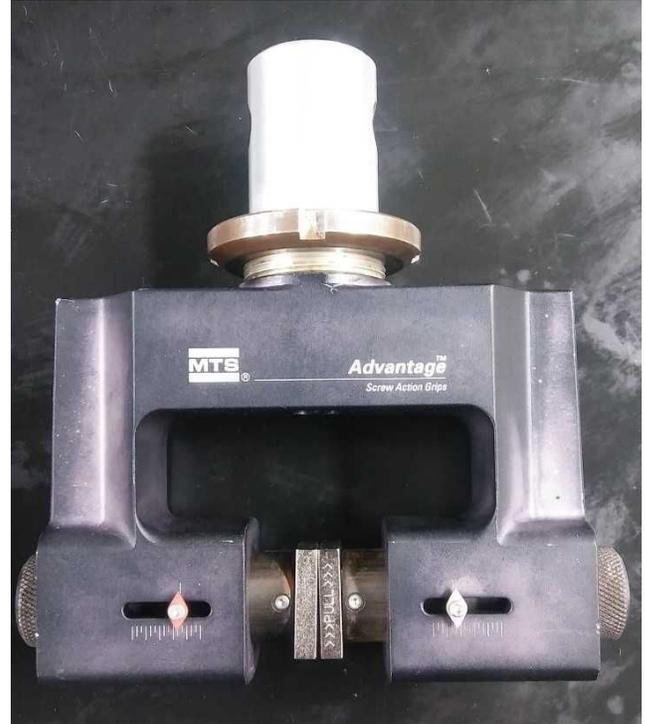
**Figure 1.** MTS clamp attachment used to hold a dowel pin inside the prototype.
