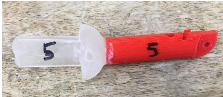
**Figure A2.** Images of three point bending samples after testing. Sample 1 failed at the interfacial bond. Sample 2, 3, and 5 failed within the bulk of the part. Sample 4 had cracks both at the bond and within the part.
