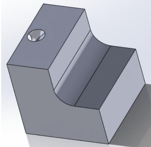
**Figure 3.** Solid view of MTS Stage adapter. The MTS Stage adaptor places the finger bridge in the line of action of the thumb grip attachment and stabilizes the prototype.
