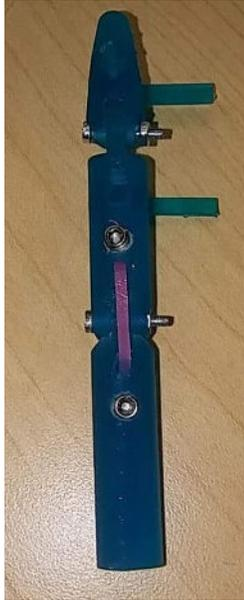
**Figure 7.** Image of prototype. Finger bridges can be seen extending laterally from the palmar side of the medial and distal segment. A rubber band is inserted on the dorsal side of the segments around the joints.
