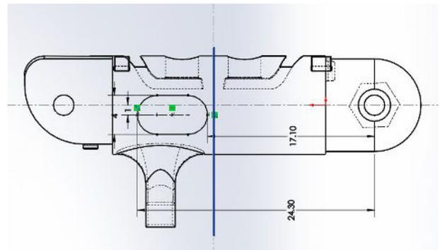
**Figure 6.** Image of the cross section of the medial segment of the prototype, showing the dowel pin slot used for MTS attachment.
