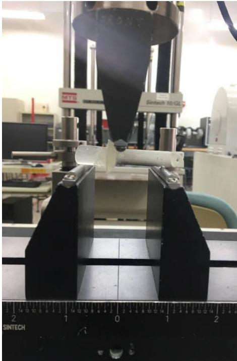
**Figure 9.** Image of three point bending setup. The piston tip was positioned as close to the interfacial bond as possible.
