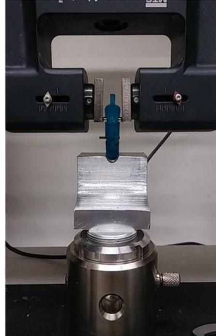
**Figure 5.** Image of the MTS setup with the clamps and MTS stage adapter with a dowel pin bending the PIP joint. Bridge is clipped.
