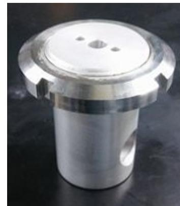
**Figure 2.** MTS base attachment with a hole for the pin. The MTS Stage Adapter is attached to the hole using an M6x1 screw.
