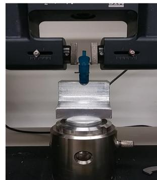
Figure 5. Setup of MTS testing with prototype.
