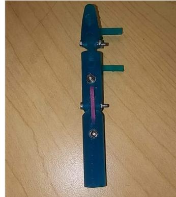
Figure 4. Printed prototype; note lack of distal elastic
