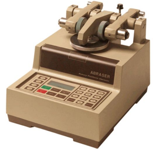
Figure 10: Rotary Platform Double Head Abrader for ASTM D3884
